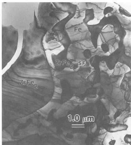
FIG. 2—Bright field (BF) of ZrFe_2 alloy showing the two types of C15 ZrFe_2 : a bulk phase designated ZrFe_2 and a high stacking fault density phase designated ZrFe_2 -SF.
