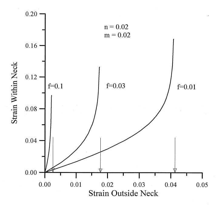
Figure 2. The development of a localized necking instability for the plane-strain deformation of cladding containing imperfections of differing severities f. Strains are maximum principal strain values and arrows denote the limit strain for each case.
