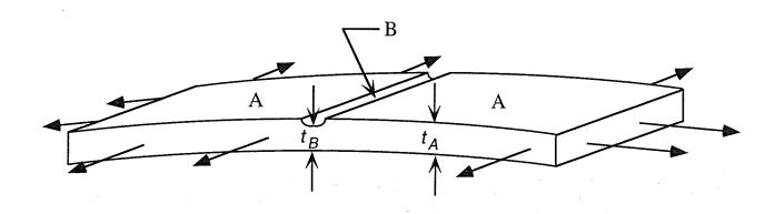
Figure 1: A schematic drawing indicating an imperfection reducing the thickness of the sheet from  $t_A$  to  $t_B$ . Plane-strain conditions are indicated during sheet extension.
