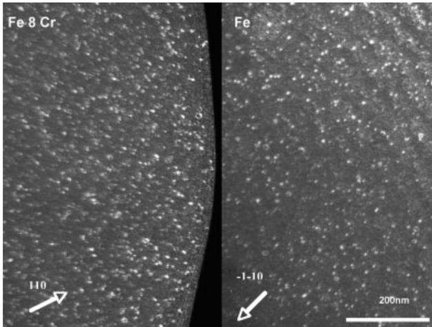
Fig. 3. Damage microstructures in bulk specimens of pure Fe and Fe-8%Cr following 1.5 MeV Fe ion irradiation at 300°C to 2.5 dpa and imaged in WBDF with  $g = \langle 110 \rangle$ .
