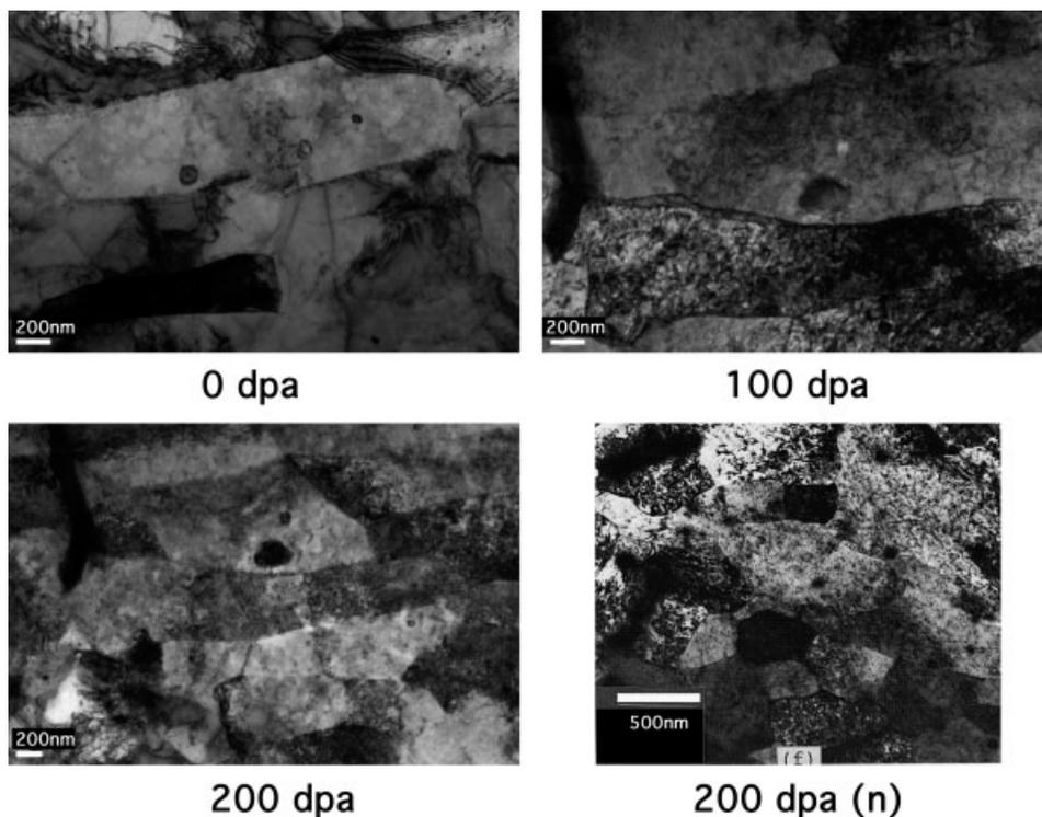
Fig. 4. Bright field images of MA957 ODS alloy irradiated in situ at 500°C with 1 MeV  $\text{Kr}^{++}$  ions (first three panels, size bar = 200 nm) and ex situ with fast neutrons at 420°C (Gelles, 1996, fourth panel, scale bar = 500 nm).
