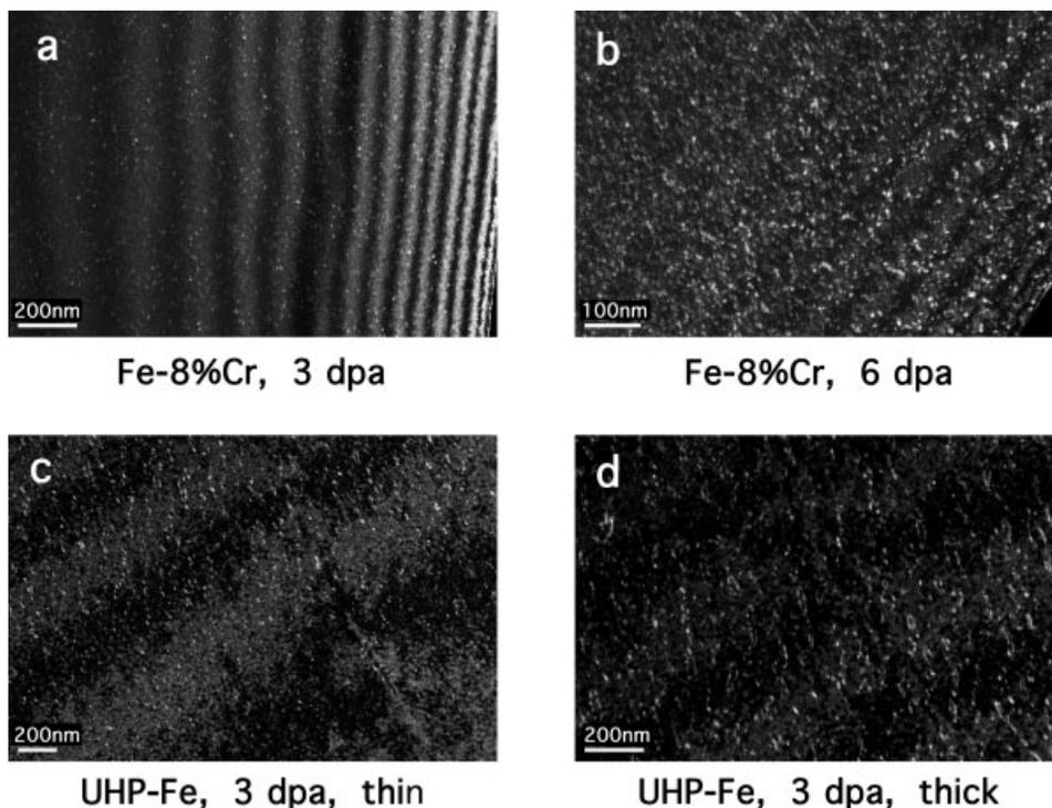
Fig. 2. Comparisons of defect microstructure in ultra-high purity (UHP) Fe and alloy of Fe with 8%Cr, irradiated with 150 keV Fe ions to given damage levels at a sample temperature 300°C. Imaging condition is weak-beam dark-field (WBDF) with  $g = \langle 110 \rangle$  ( $g, 4g$ ).
