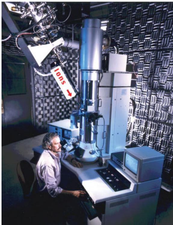
Fig. 1. IVEM-tandem in situ user facility: Hitachi 9000 NAR microscope, ion beam interface to microscope, and Dr. Charles W. Allen (responsible for installation and principal investigator, now retired). [Color figure can be viewed in the online issue, which is available at [www.interscience.wiley.com](http://www.interscience.wiley.com).]
