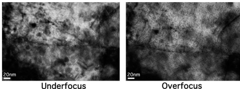
Fig. 5. Bright field defocus images of small (1–2 nm) voids in MA957 ODS alloy irradiated in situ at 500°C with 1 MeV  $\text{Kr}^{++}$  ions to a dose of 200 dpa. Scale bar = 20 nm.
