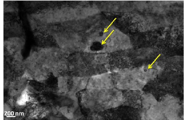
Fig. 3. Bright Field TEM micrograph of MA957 irradiated with 1 MeV Kr ions at 500°C to ~200 dpa. Despite a large amount of damage the alloy retains its grain morphology after 200 dpa and the large precipitates remain crystalline.
