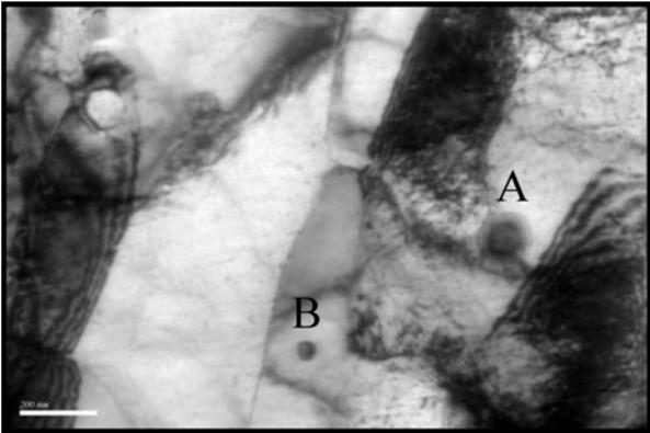
Fig. 2. Bright Field TEM micrograph of MA957 irradiated with 300 keV Fe ions at 25°C to ~18 dpa: some oxide particles exhibit a halo, indicating dissolution at the surface (particle A), while other oxide particles are more stable (particle B). The difference in behavior most likely comes from the difference in local chemical composition.
