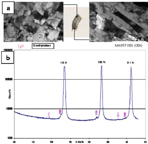
Fig. 1. (a) Bright Field TEM images of the grain microstructure in MA957 ODS steel in transversal direction (left) and (right) circumferential direction and (b) XRD spectrum from 15keV synchrotron irradiation showing Fe matrix peaks and oxide peaks.
