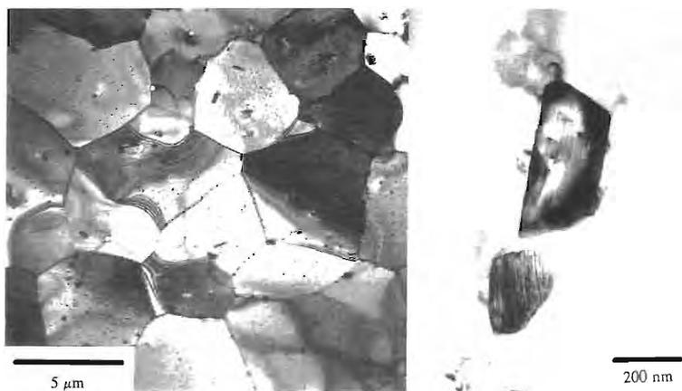
**Figure 7-7.** Typical distribution of second phase precipitates  $Zr(Cr, Fe)_2$  and  $Zr_2(Ni, Fe)$  in recrystallized Zircaloy.
