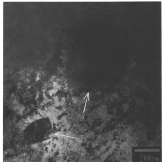
Fig. 5. Large microcrystalline oxidized precipitate (A) near a small unoxidized one (B) located in the bulk of a 4\ \mu\text{m} thick oxide layer (at about 1\ \mu\text{m} from the metallic interface).
