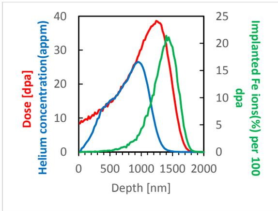
**Fig.1** Damage profile (red) and ion implantation (green) as calculated by SRIM for 5 MeV Fe atoms into Fe21Cr32Ni model alloy. Helium implantation is shown with blue line.
