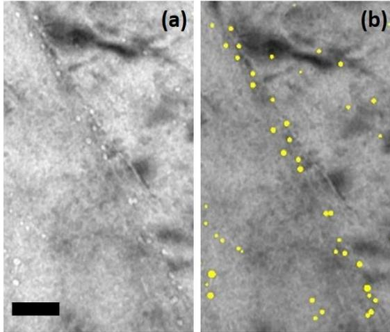
**Fig. 3 (a)** Dual beam irradiated 21Cr32Ni alloy microstructure showing cavities preferentially formed along the grain boundary, **(b)** voids in (a) are highlighted for better visibility.
