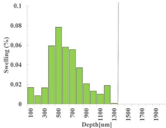
**Fig. 4** Percent swelling vs. depth profile in dual beam irradiated 21Cr32Ni austenitic alloy.
