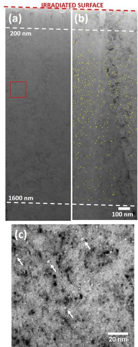
**Fig. 2** (a) Cavity distribution in 21Cr32Ni model alloy after dual beam irradiation at  $\sim 440^\circ\text{C}$  dose in dpa, (b) cavities in (a) are highlighted for better visibility, (c) High magnification image of the cavities observed at  $\sim 600$ nm target depth indicated with red box in (a)
