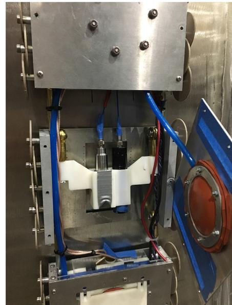
Fig. 7. The LIBS optics holder mounted in the PRINSE train car. Operation of this system was tested once fully inserted into a simulated canister channel.
