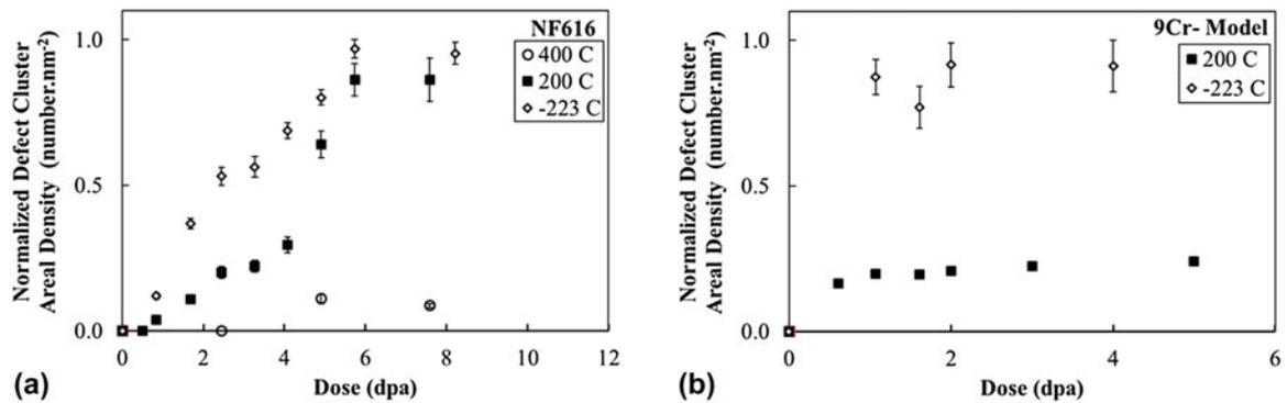
FIG. 24. Normalized defect cluster areal density of (a) NF616 and (b) 9Cr-model alloys as a function of dose. The defect cluster density is normalized to the highest value acquired (5.5 dpa at  $-223$  °C for NF616 and 2 dpa at  $-223$  °C for 9Cr-model alloy), plus the error bar.<sup>89</sup>
