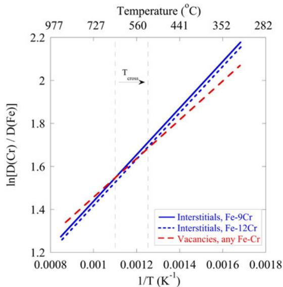
FIG. 7. Diffusion coefficient ratios of Cr to Fe for vacancies and interstitials in bcc Fe–Cr binary alloys. Crossover temperature,  $T_{\text{cross}}$ , decreases for increasing bulk Cr content. Below  $T_{\text{cross}}$ , Cr interstitial diffusion dominates, causing Cr enrichment. Above  $T_{\text{cross}}$ , Cr vacancy diffusion dominates, resulting in Cr depletion.
