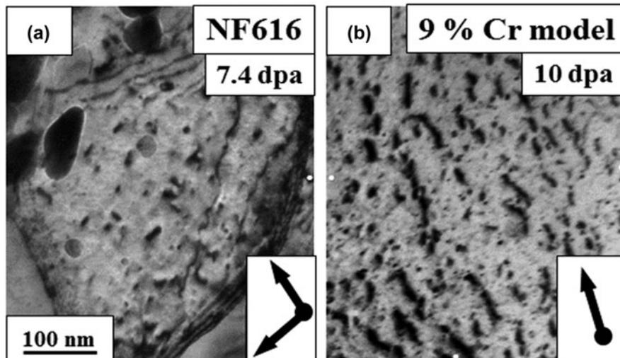
FIG. 23. Bright-field transmission electron micrographs of extended defects observed in NF616 and 9Cr-model alloys under 1 MeV Kr irradiations performed at 400 °C (a) and 25 °C (b), respectively.<sup>89</sup>
