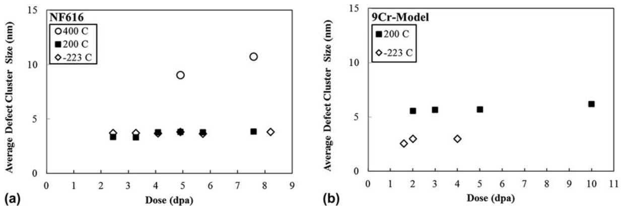
FIG. 25. Average defect cluster size of (a) NF616 and (b) 9Cr-model alloys as a function of dose.<sup>89</sup>
