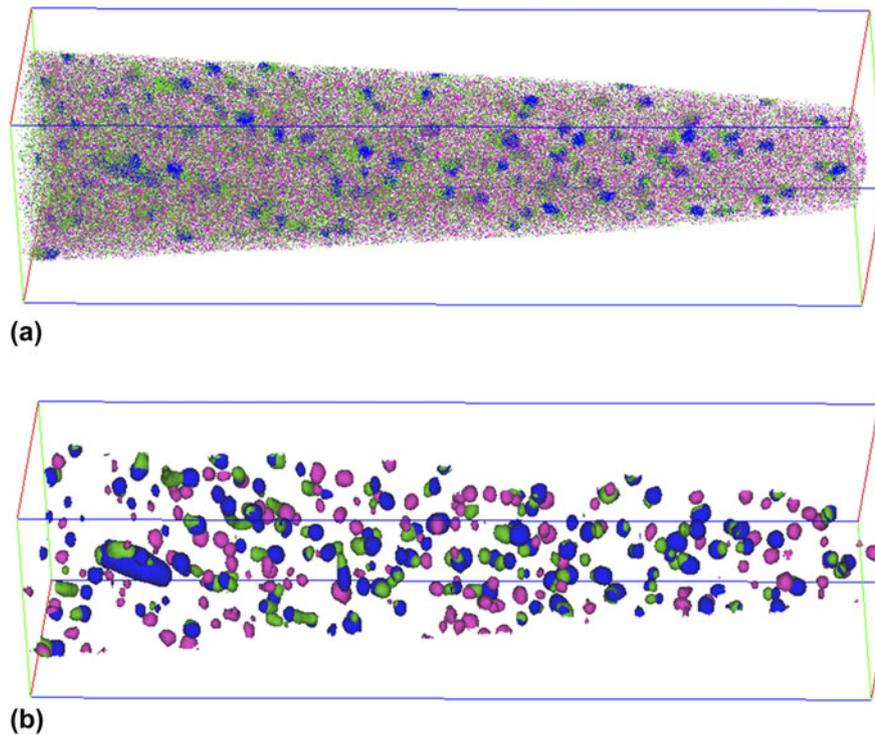
FIG. 11. APT image of a tip from HCM12A irradiated with 2 MeV protons to 7 dpa at 400 °C containing NSMPs, CuRPs, and CrRPs. (a) Ni (green), Cu (blue), and Cr (pink) atom maps. (b) NSMPs (green), CuRPs (blue), and CrRPs (pink) highlighted using isosurface plots. The dimensions of the box are  $250 \times 63 \times 63 \text{ nm}^3$ .
