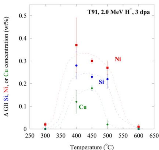
FIG. 2. Temperature dependence of Si, Ni, and Cu RIS in alloy T91 irradiated with 2.0 MeV protons to 3 dpa, showing enrichment between 400 and 500 °C and RIS suppression at 300 and 600 °C.
