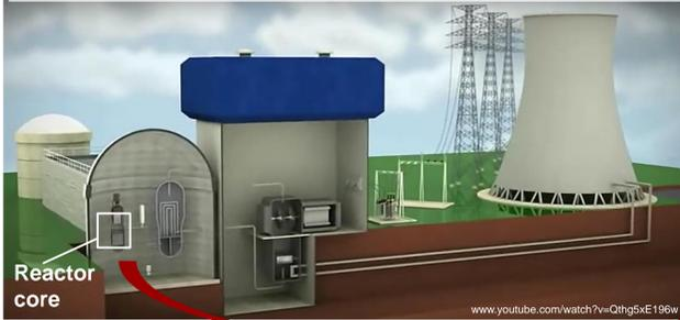
Energy is created in the reactor core using 4 m long fuel rods.
